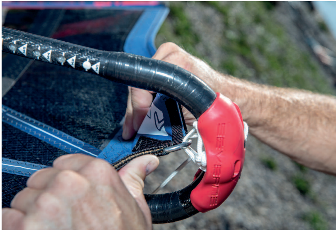
Above: Casually adjusting your boom height can throw your outhaul setting out, so any boom height change must be matched by adjusting the outhaul
