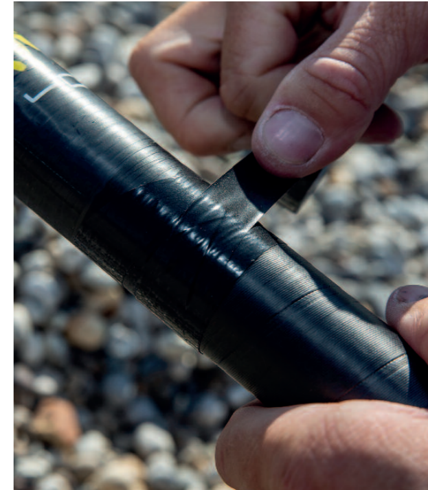
Above: Taping mast sections tightly can prevent separation inside the luff tube during rigging
