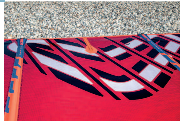
Above: It's all in the detail. Spot the difference between these two photos. One has a loose and reactive leech thanks to correct downhaul whereas the other has a tight and choked leech thanks to too little downhaul
