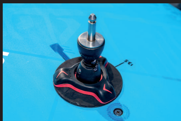
Marking your mast track is the first step to standardising your tuning and understanding the relationship between mastfoot, boom height and outhaul
