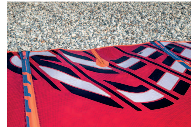
Above: It's all in the detail. Spot the difference between these two photos. One has a loose and reactive leech thanks to correct downhaul whereas the other has a tight and choked leech thanks to too little downhaul
