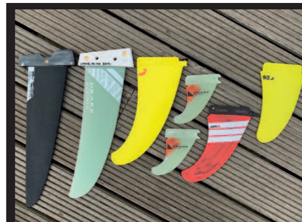
A range of fin types and shapes: (from left to right): slalom/race, freeride, freewave single, freewave thruster setup (tri fins) and freestyle
