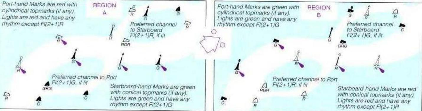
A preferred channel buoy may also be a pillar or a spar. All preferred channel marks have three horizontal bands of colour.
